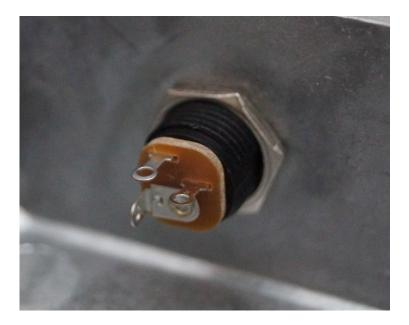
Then, solder the three wires from the DC connector in the board to the DC jack as follows:
