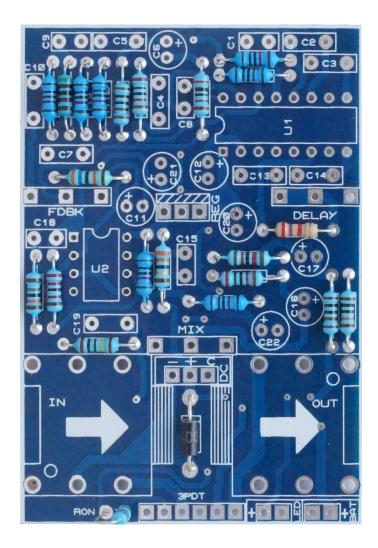
Place the resistors and diodes. If you have troubles reading the values, check out our <u>"Reading Part Values"</u> tutorial.
